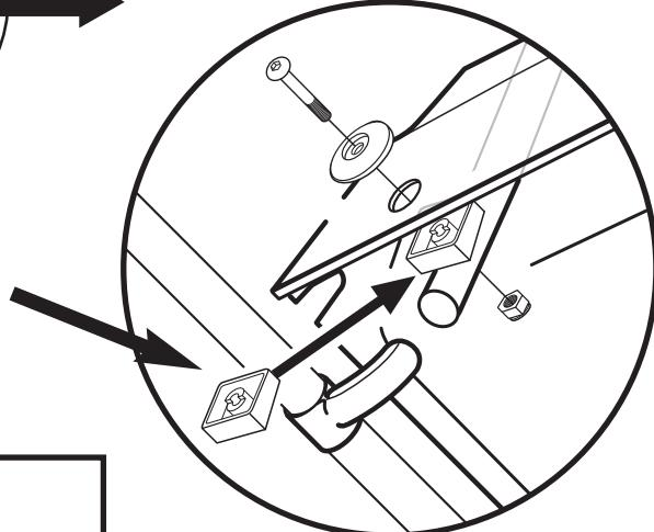
**Bolt Tightening Guide**
